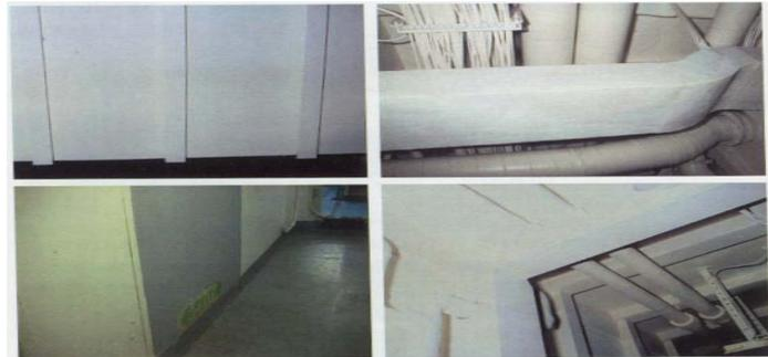
Temp Coat applications onboard USS Bonhomme Richard (LHD 6) (top) and USS Rushmore (LSD 47) (bottom) include bulkheads, overheads and ducting.
