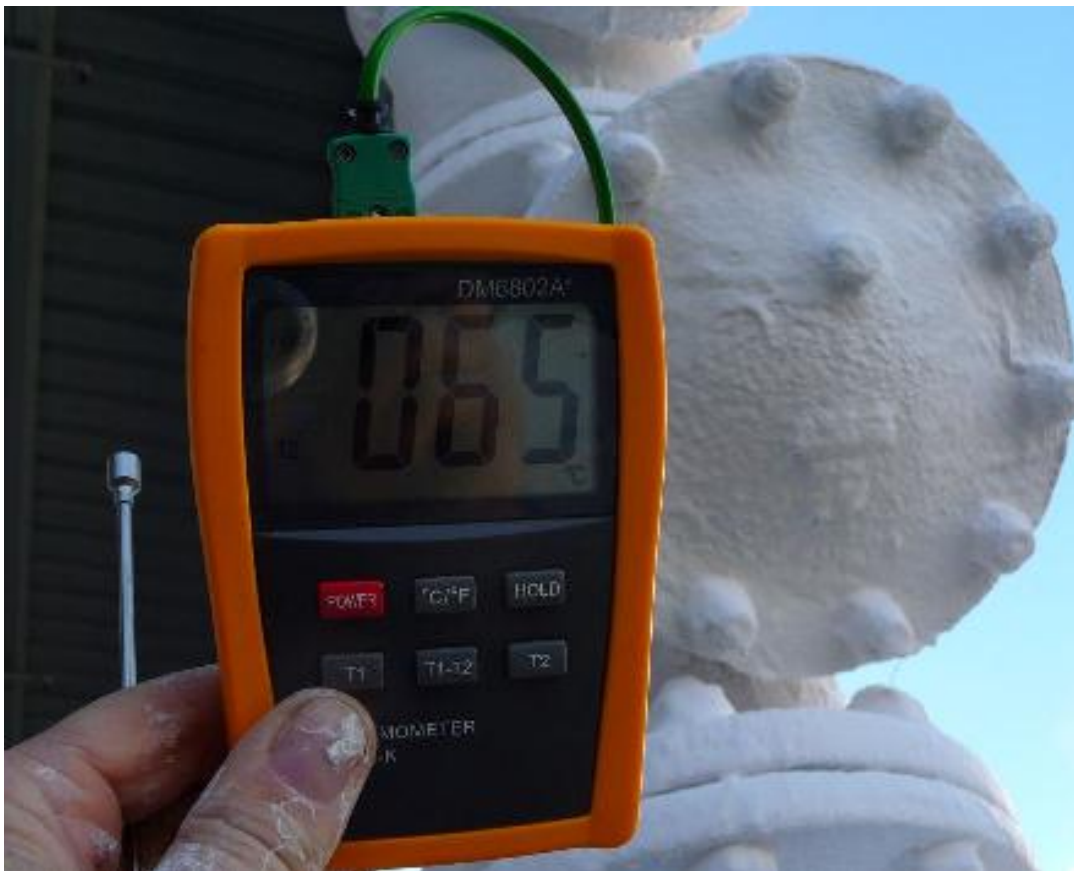
TEMP-COAT®101 insulation Coating applied at 3mm reduced temperature to 65°C
